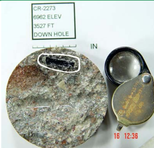
Figure 2. A carbonized wood fragment, from the Cresson surface mine, is circled in this core sample. This impressive sample was sliced from a piece of NQ-sized drill core (just under 2 inches in diameter). Image courtesy of the Cripple Creek and Victor Gold Mining Company.
